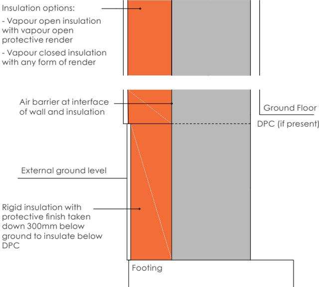
**Figure C.8** - Insulation strategy for solid wall - external wall insulation (EWI)
