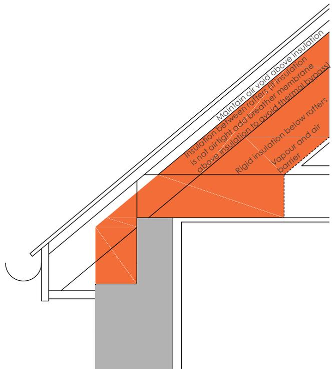
**Figure C.13** - Insulation strategy for cathedral roof insulated between and below rafters
