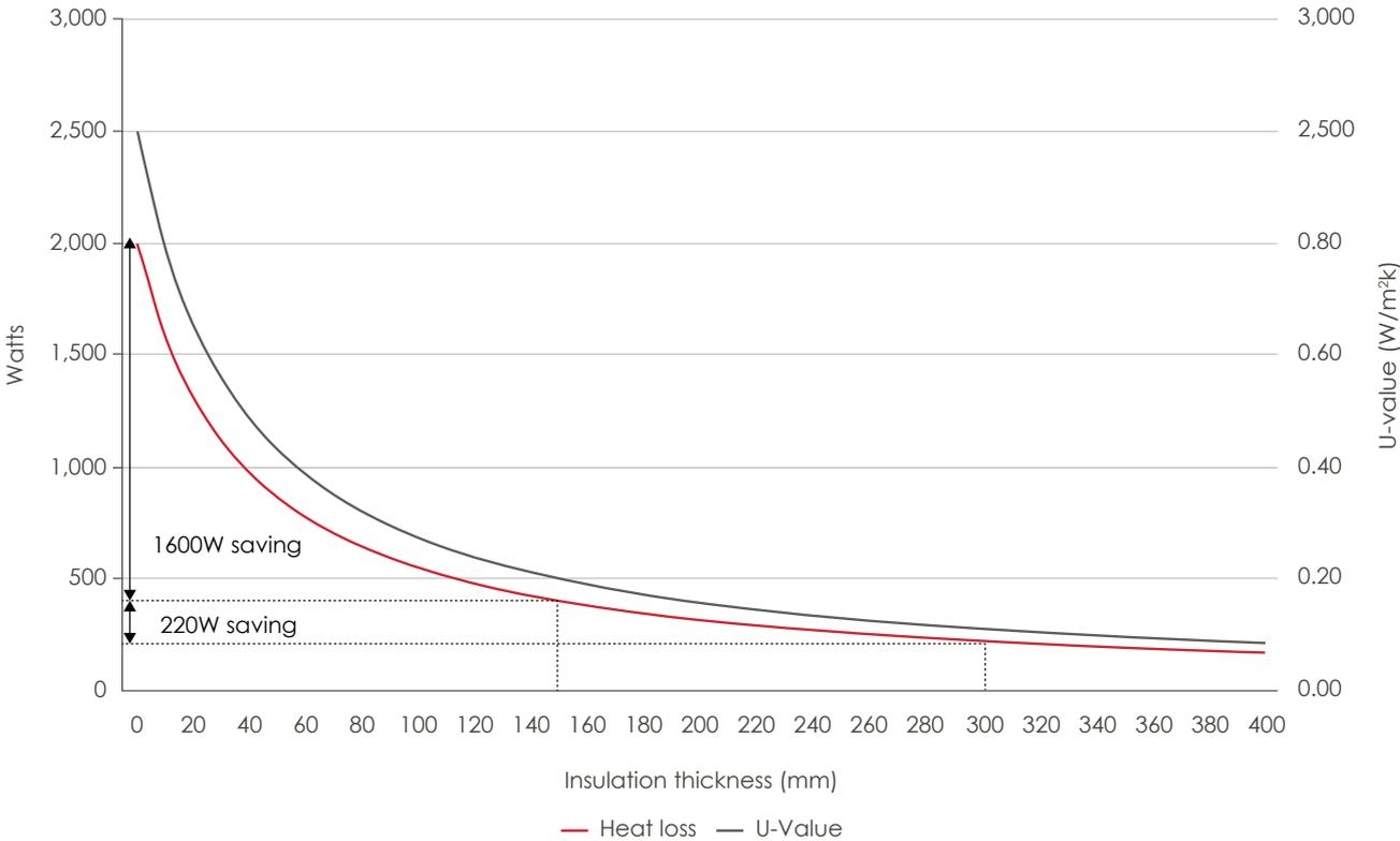
Figure G.1 - Diminishing returns for the amount of insulation being applied to a 100m<sup>2</sup> solid wall with external temperatures at 0°C
