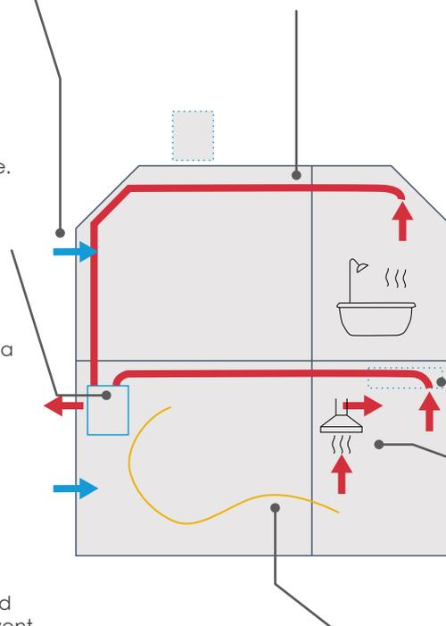
Figure D.2 - Centralised constant extract ventilation with demand control (dcMEV)
