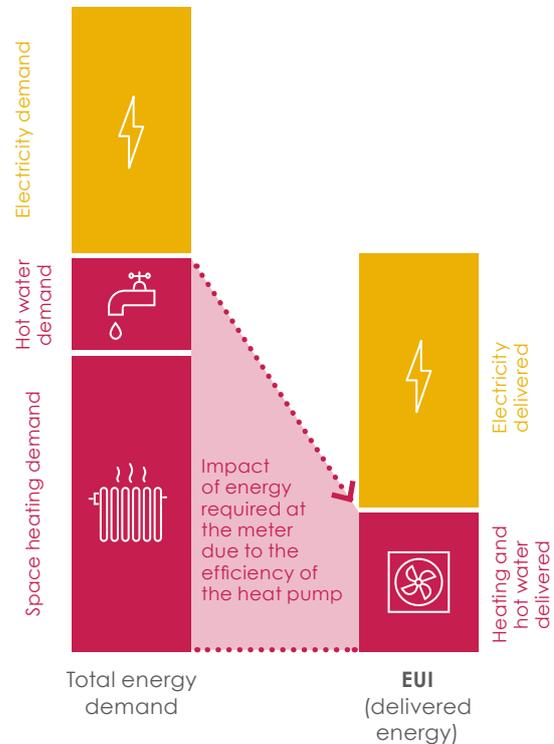
Figure 3.4 - Relationship between energy demand and EUI when using a heat pump.
