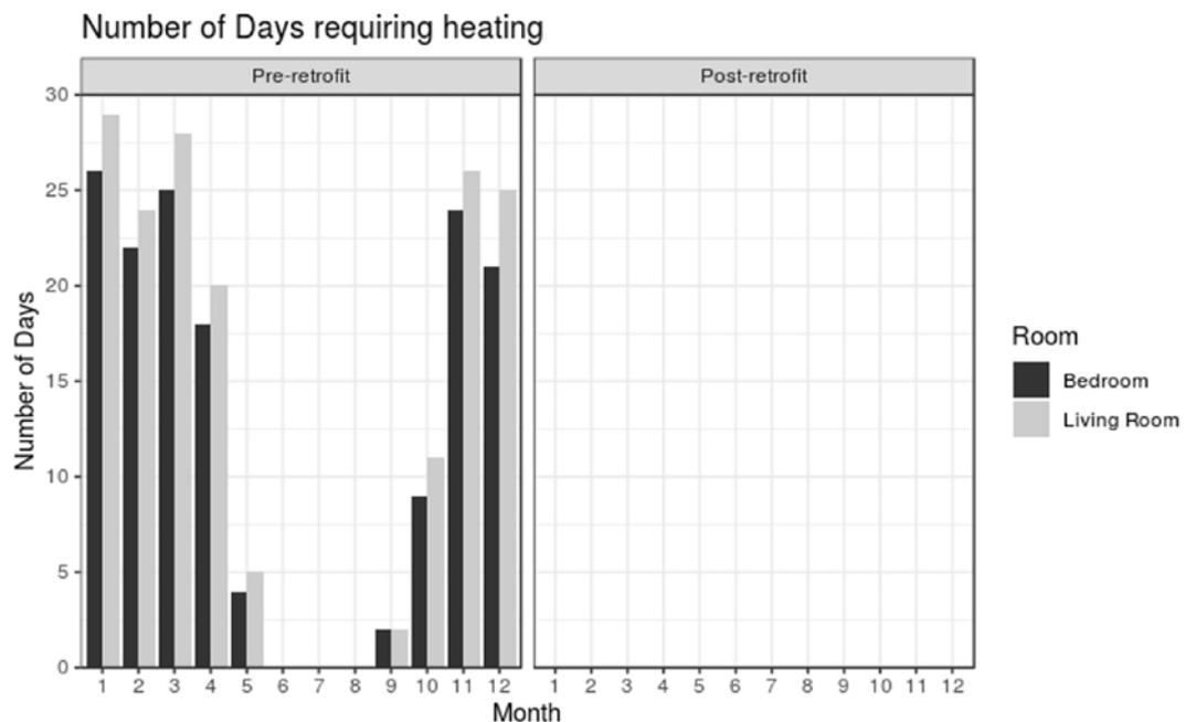
**Figure 6.16** - Bar graph showing hypothetical performance under a TMY (Typical Meteorological Year). Showing the number of days that would typically require some form of heating in order to maintain 18°C<sup>6,6</sup>. This graph shows that no active space heating is required post-retrofit to maintain 18°C.
