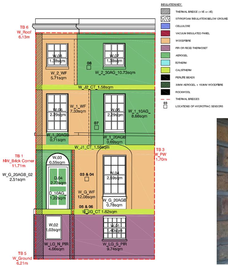
Figure 6.39 - Schematic of types of insulation to rear elevation, Arboreal Architecture
