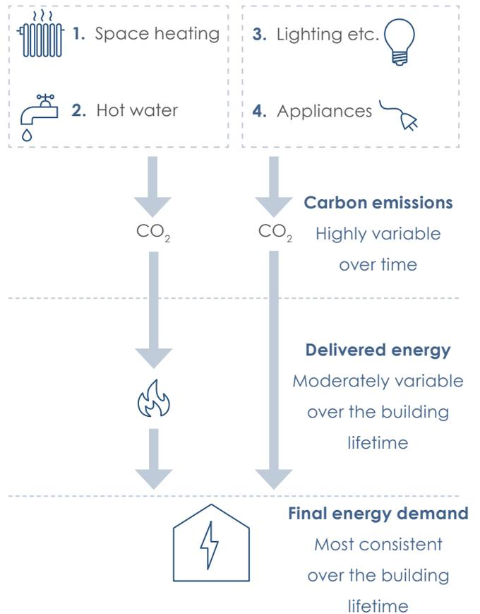
Figure A.4 - How variable is the chain of delivery of energy to the building
