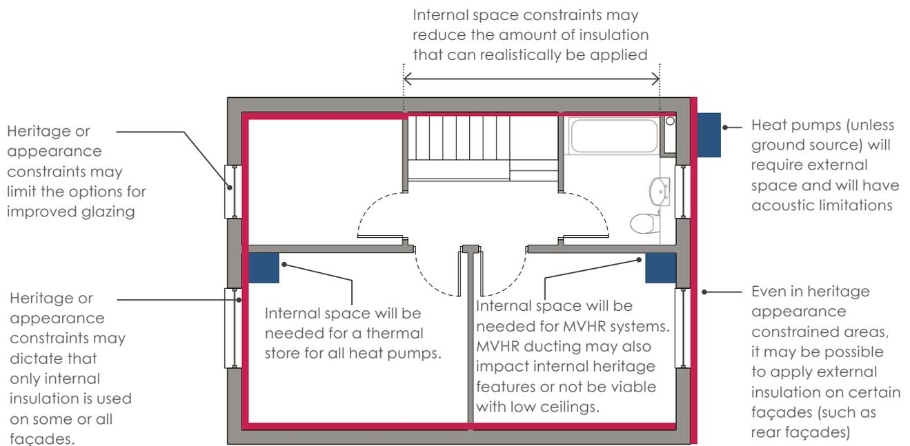
Figure 3.8 - Constraints on retrofit scope.
