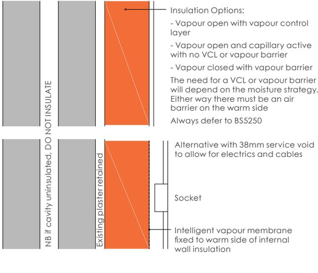
**Figure C.11** - Insulation strategy for cavity wall - internal wall insulation (IWI)
