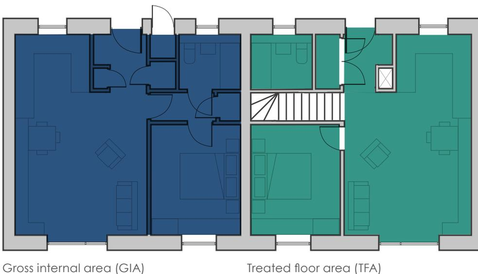
**Figure 2.8** - Illustrative difference between GIA and TFA floor area measurements
