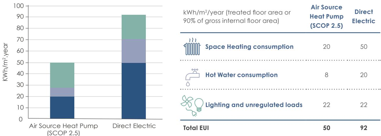
**Figure 4.2** - Graph and table showing comparison of EUI for an air source heat pump versus direct electric for the same dwelling
