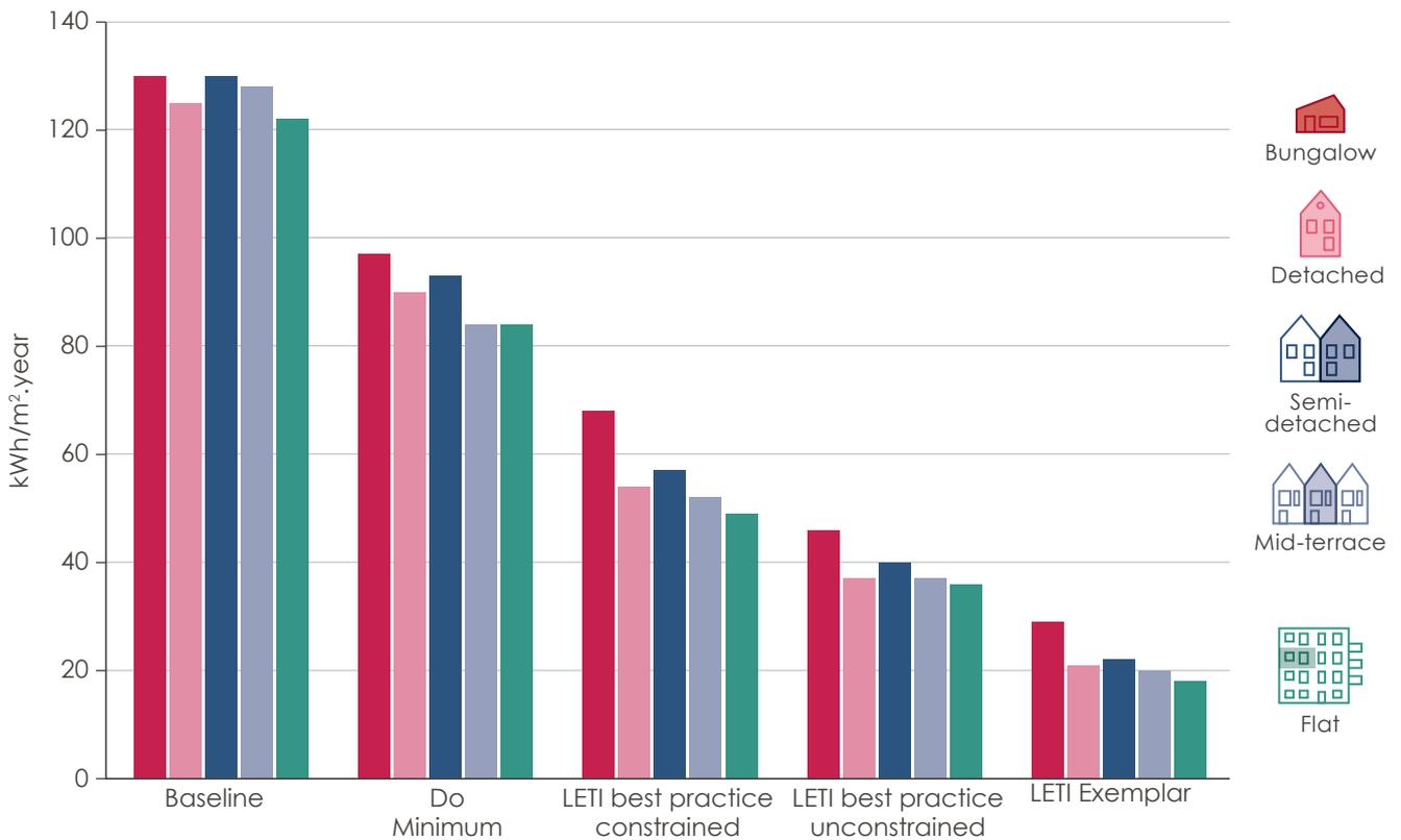
Figure 3.10 - Effect of varying retrofit scenarios on space heating demand (the energy needed to heat the space, independent of type of heat source used), by building form.
