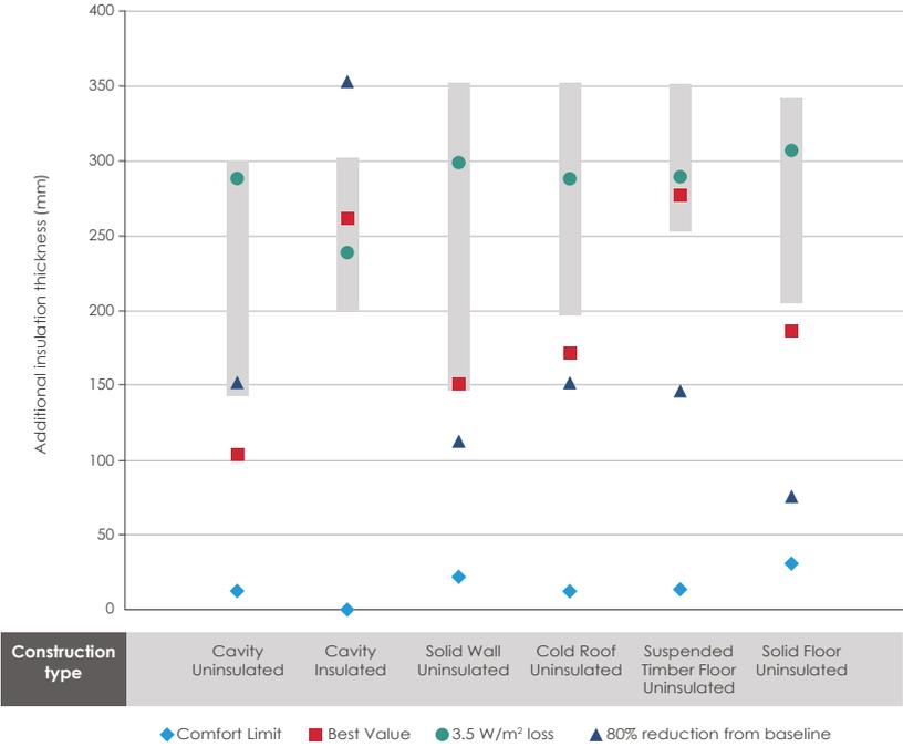
Figure G.8 - Thickness of additional insulation by baseline construction (ext temp -10 Degrees Celsius)
