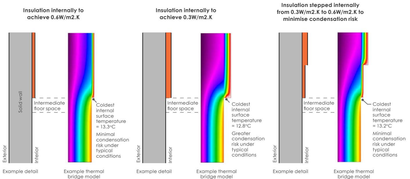
Modelling parameters: 0°C externally, 20°C internally. Brick conductivity 0.77W/m.K; insulation conductivity, 0.04W/m.K
